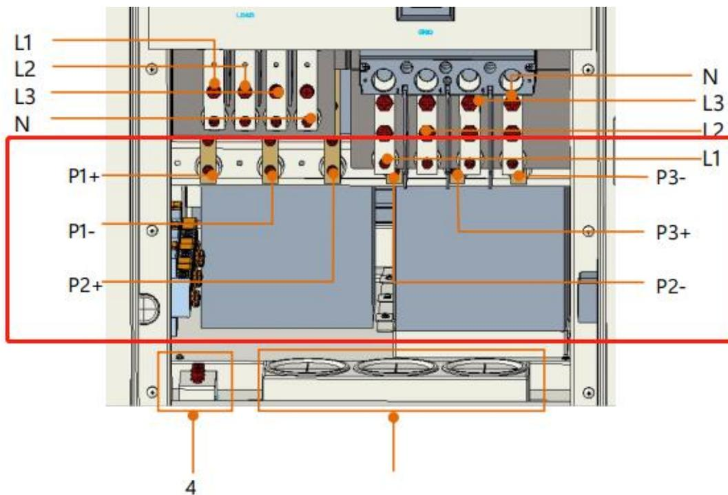
Each MPPT corresponds to one P+ and one P -, and this project is equipped with three 50kW-MPPT modules for each DH200F
