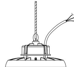
3. Ensure the terminal connection is made inside a suitable IP65 rated junction box. (not included)
