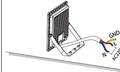
3-Ensure the terminal connection is made inside a suitable IP65 rated junction box. (not included)
