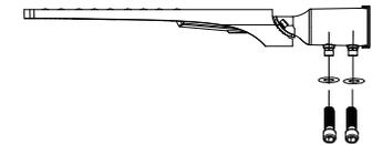
2. Connect the Main Line to the power wire of the lamp
