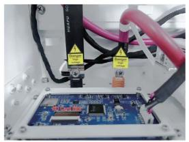
Note: When inserting the SD card, unplug the battery power cord and manually turn the air switch to the off position.
