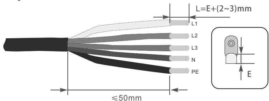
Step 2. Make the cable and crimp the OT terminal.
