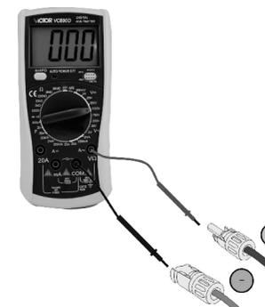
Check the positive and negative polarity of the PV strings, and connect the PV connectors to the right terminals. Serious damages to the inverter and connector over temperature may occur.
