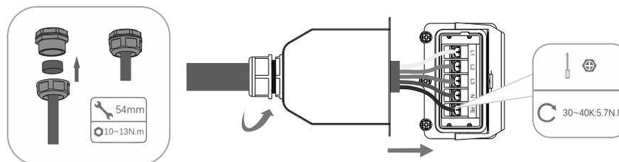
Step 4. Secure the junction box, fasten the buckle, and secure it with screw.
