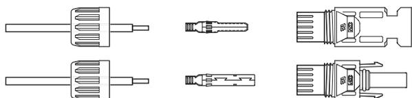
▲ Figure 4.8 Disassemble the Connector Cap nut
