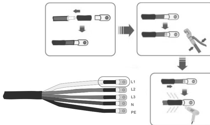
Step 3. Follow the instruction and secure the cable to corresponding terminals.
