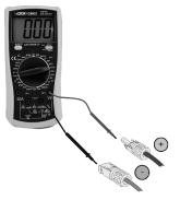
Check the positive and negative polarity of the PV strings, and connect the PV connectors to the right terminals. Serious damages to the inverter and connector over temperature may occur.
