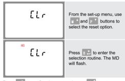
Press E Lato confirm the reset and press V/I to return to the main set up menu.
