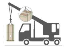
Before hoisting, check whether the pallets and cartons are damaged and whether the hoisting ropes are strong and firm. When the lifting is about to hit the ground, one person on each two side should upright the carton gently on the relatively flat position of the project ground.
