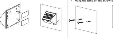
· Take out expension bolt and screws, fix them into installation surface according to holes on the back of the lamp; leave a little space between the screws and the installation surface.
