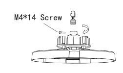
Take out the lifting ring from the accessory bag and screw it into the top of the power supply. The lifting ring of the Edison power supply is M10 and the maximum torque value is 19NM. Then screw in the M4\*14 screw from the side, the maximum torque value is 2.2NM.
