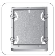
Make sure the filters are installed in position. 4 To install the front panel, place the bottom Turn the buckles to fix the filters.
