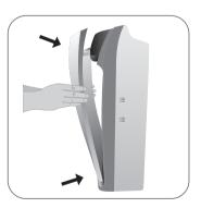
part into the host buckle and close the front panel. The front panel will be held by in-built magnets.
