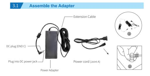
A.Connect the power adapter to the power cord as shown in Figure (1)
