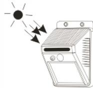
1. Choose a place to make sure the solar panel can get full sunlight. (In human sensor mode, it should be mounted within three meters.)
