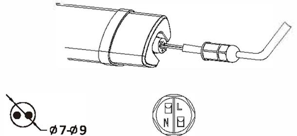
Outside the connection wire diameter shall apply:2G1mm~2G1.5mm
