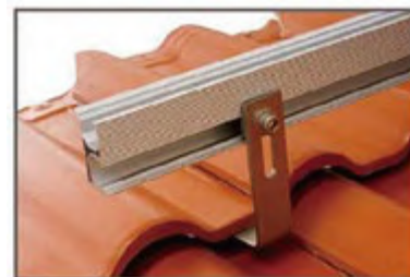
Step 2: Fix solar rail on tile hook and lock tightly by M8x25mm T module set.
