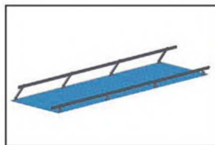
Step 2: Fix solar rail on adjustable front leg and rear leg
